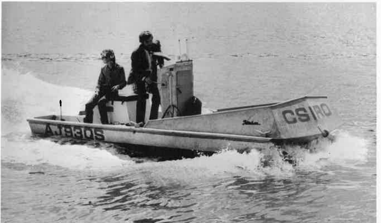
THE "JET-BOAT". A prop-less craft for shallow water work.
